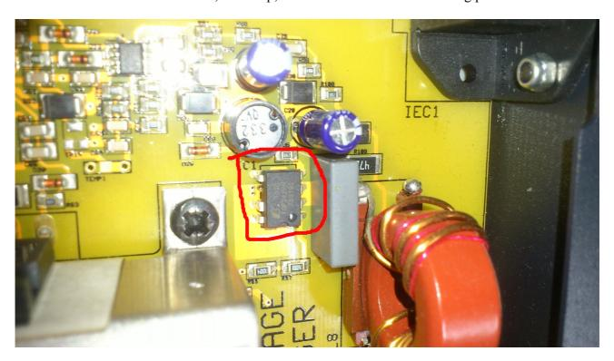
If the device fails, the amp will: power on normally, then after about 10 to 30 minutes, the amp will shut down completely, no front panel lights, no fans. Power down occurs when the TOPSwitch IC reaches 125 degrees C. Allowing it to cool will restore operation of the amplifier. The normal running temperature of this IC is around 75 to 85 degrees.
