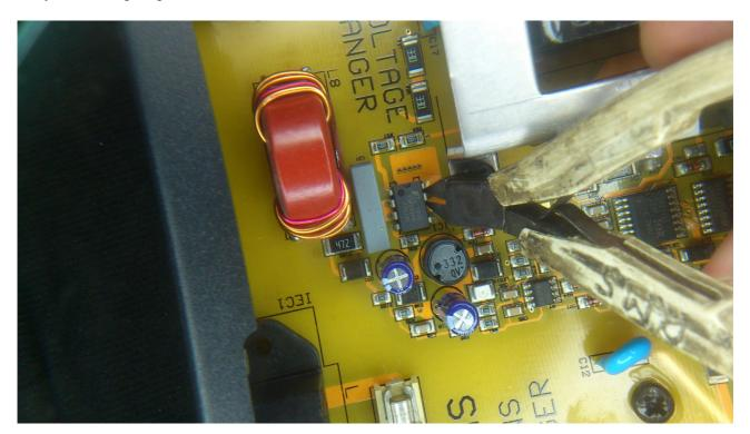
Step 2: (no image) With a soldering iron, heat the remaining part of each chip leg close to the bard surface for around 5 seconds. Using tweezers or fine pliers, grasp the leg and remove it from the board. You will need a little more heat on the legs on the "groundplane" sections, but all should come out fairly easily. We use lead-free solder, so use a hot tip on your iron.
